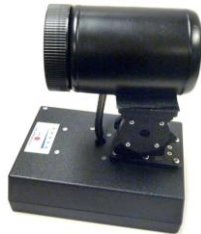
Figure 4: The Note-Taker 2.0 PTZ camera
