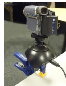
Figure 2: The Note-Taker 1.0 PTZ camera
