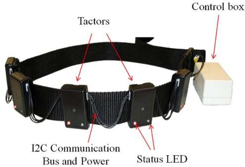
Fig. 1. Haptic belt harness and tactor modules.
