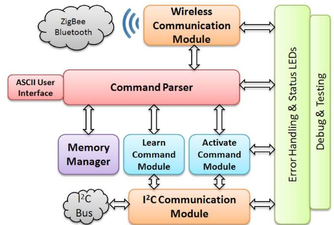
Fig. 3. Main controller firmware implementation.
