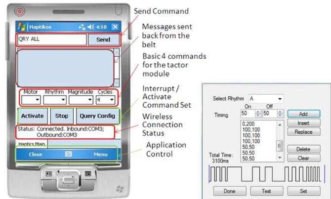
Fig. 5. (a) GUI on a portable platform. (b) TRS design interface.
