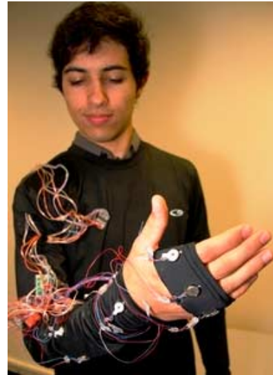
Figure 3. A user demonstrating our haptic suit for motor learning. Photo credit: Jessica Slater/ ASU.
